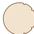
½ bastone liscio e ½ bastone rigato Pole is ½ smooth and ½ reeded
